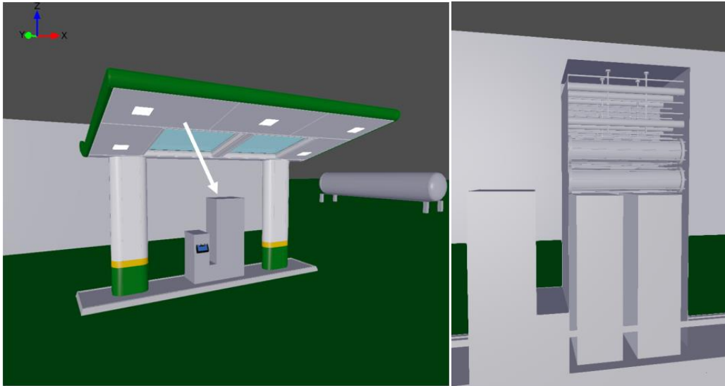
Figure 3-4: Dispenser cabinet indicated by white arrow (left). Dispenser cabinet with front wall removed (right).
